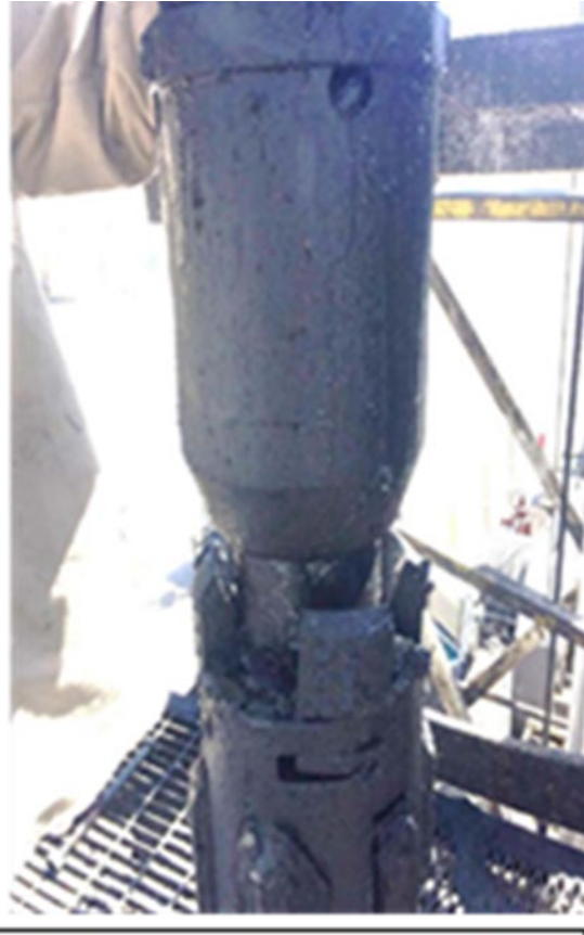
Figure 3: Well 58-32 packer damage
